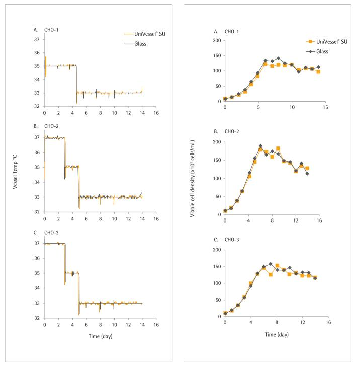
Figure 2: Comparison of on-line vessel temperature control during (a) CHO-1 (b) CHO-2 and (c) CHO-3 processes between UniVessel® SU and Applikon glass vessels with either a single or dual temperature shift
