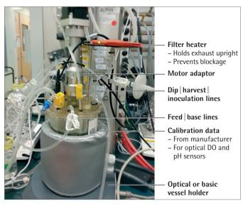
Figure 1: Set up of water jacketed 2L UniVessel® SU
