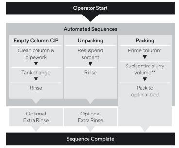
Figure 1: Packing | Unpacking | CIP Sequence Overview
