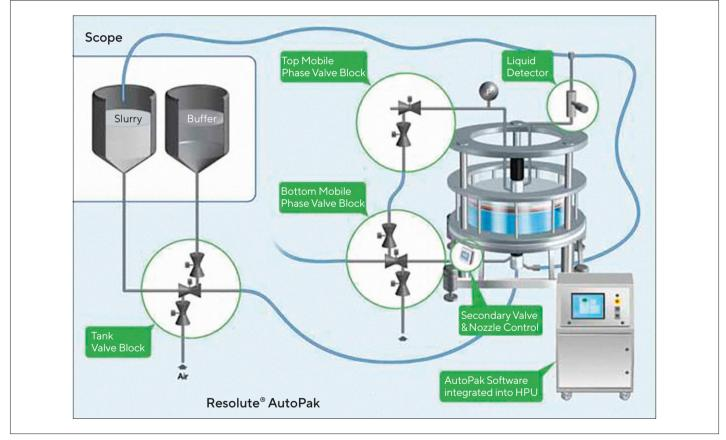
Figure 2: Typical AutoPak System Schematic
