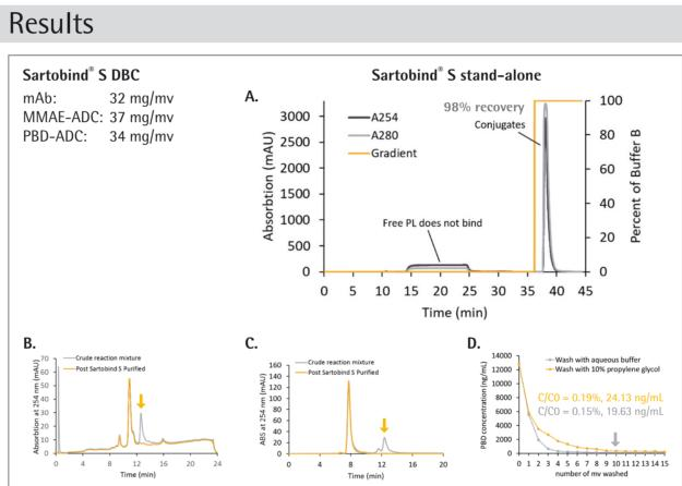
Figure 2: (A) Removal of residual PBD using Sartobind<sup>®</sup> S in stand-alone model. The quenched reaction mixture (gram scale) was loaded to a 150 mL Sartobind<sup>®</sup> S membrane, then washed with 10 mv binding buffer prior to elute. (B) HIC and (C) SEC profiles showing the removal of free PBD dimer. (D) LC-MS method showing PBD dimer removal efficiency with Sartobind<sup>®</sup> S.
