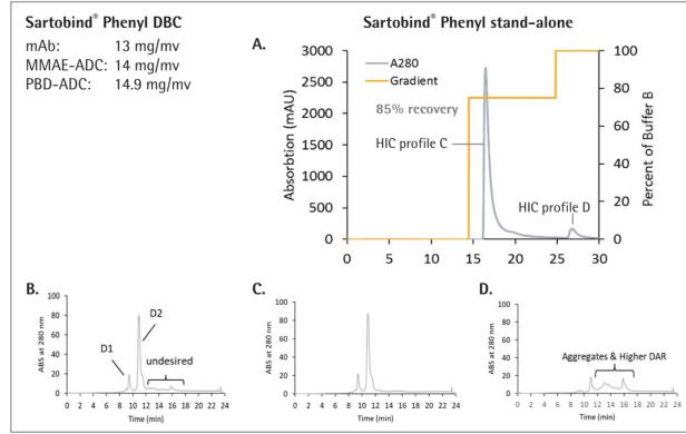
Figure 3: (A) Purification of engineered Cysteine-mAb-PBD ADC using Sartobind<sup>®</sup> Phenyl in stand-alone model. The Sartobind<sup>®</sup> S purified material (gram scale) was loaded to a 150 mL Sartobind<sup>®</sup> Phenyl membrane, then targeted and undesired ADC species were eluted sequentially. (B) HIC profile of Sartobind<sup>®</sup> S purified ADC. (C) HIC profile of Sartobind<sup>®</sup> Phenyl purified ADC. (D) Aggregate and higher DAR species was in the final wash step.
