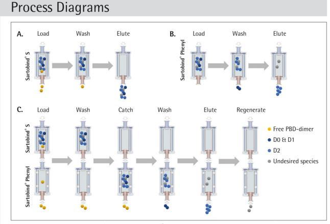
Figure 1: Process diagram. (A) Bind | Elute using Sartobind<sup>®</sup> S to remove residual payload, and (B) Bind | Elute using Sartobind<sup>®</sup> Phenyl to remove aggregate in stand-alone model; (C) Simplified process to purify target ADC with Sartobind<sup>®</sup> S and Phenyl in tandem model.
