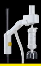
Cell Plus filter with 15 kDa cut off removes endotoxins, RNase/DNase
