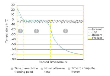
Figure 1: Celsius® FFT 2L typical freezing temperature profile
