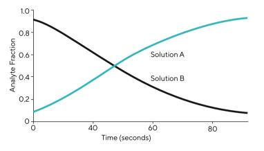
Figure 2: Time course charting the fraction of each solution as it passes through the flow cell. At the beginning of the injection, the solution almost entirely consists of solution B (the competitor molecule), however as the injection progresses, it is gradually replaced by solution A (the analyte + competitor molecule), until the final stages of the injection, which consists primarily of solution A.
