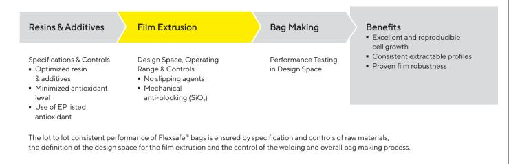
Figure 11: Quality by design principles for the development and validation of Flexsafe® bags.
