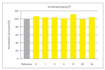
Figure 6: Cell growth testing of  ${\sf Flexboy}^{\circledast}$  against glass bottle reference during the three-year shelf life.
