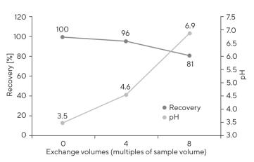
Figure 3: Washing of a graphene oxide dispersion (100  $\mu$ g/mL) using a Vivaflow<sup>®</sup> TFF cassette (RC membrane) with a MWCO of 100 kDa to reach a neutral pH. Recovery of graphene oxide and the pH of the dispersion are shown as a function of the exchange volume of the wash solution as a multiple of the feed volume of 250 mL (n = 2).
