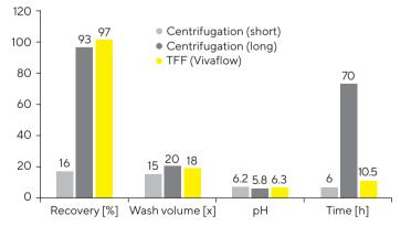
Figure 2: Comparison of methods for washing a graphene oxide dispersion (400 mL, 100  $\mu$ g/mL) with respect to the recovery of graphene oxide after the washing process and the total time required to reach a neutral pH (n = 1). Centrifugation (short) = 7 cycles with 1-hour steps each, Centrifugation (long) = 7 cycles with 10-hour steps each and TFF (Vivaflow<sup>®</sup>) by continuous buffer exchange.
