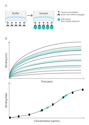
Note. (A) Quantitation assay workflow starts with equilibration of the Octet® AAVX Biosensors in the assay buffer (Buffer) followed by quantitation of AAV capsid (Sample). (B) Schematic representation of quantitation analysis of AAV standards and unknown samples on the Octet® BLI platform.
