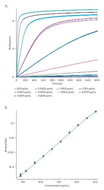
Note. (A) AAV8 serotype dose response for capsid titer within the biosensor dynamic range of 7.62E8–1.0E13 vp/mL. (B) AAV8 capsid titer standard curve calculated using 4PL (weighted Y) fitting model (log scale applied to illustrate calibration curve accuracy at the low end). The Octet® Sample Diluent was used as the assay buffer.
