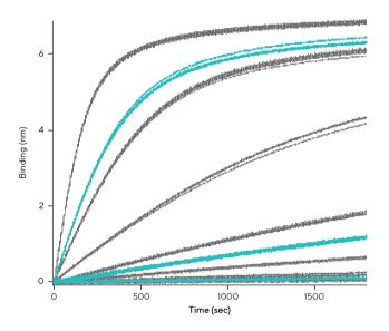
Note. The Octet<sup>®</sup> Sample Diluent was used as the matrix and all samples were analyzed in quadruplicate (binding curves corresponding to Standard Samples (gray) and Spiked Samples (teal)).
